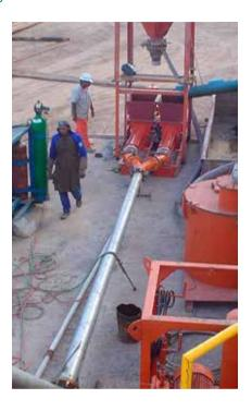
NETZSCH, the global leader in progressing cavity pump technology and sales has produced a cuttings pump to improve the solids control of the drilling fluid recovery of the VCD. This pump makes it possible to efficiently transfer drill cuttings from the shaker or from a holding vessel to the VCD.
