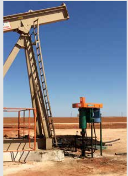
The NETZSCH Artificial Lift system suggested for a cotton field that had height restrictions due to irrigation equipment, the required flow rate and the best cost for the project.
