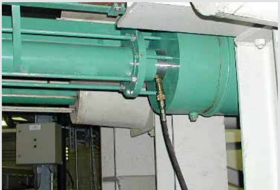
Integrated rotor/stator replacement system with inflatable shut-off (or seal-off) bladder to isolate hopper contents allows for the exchange (or repair) even with a full silo.
