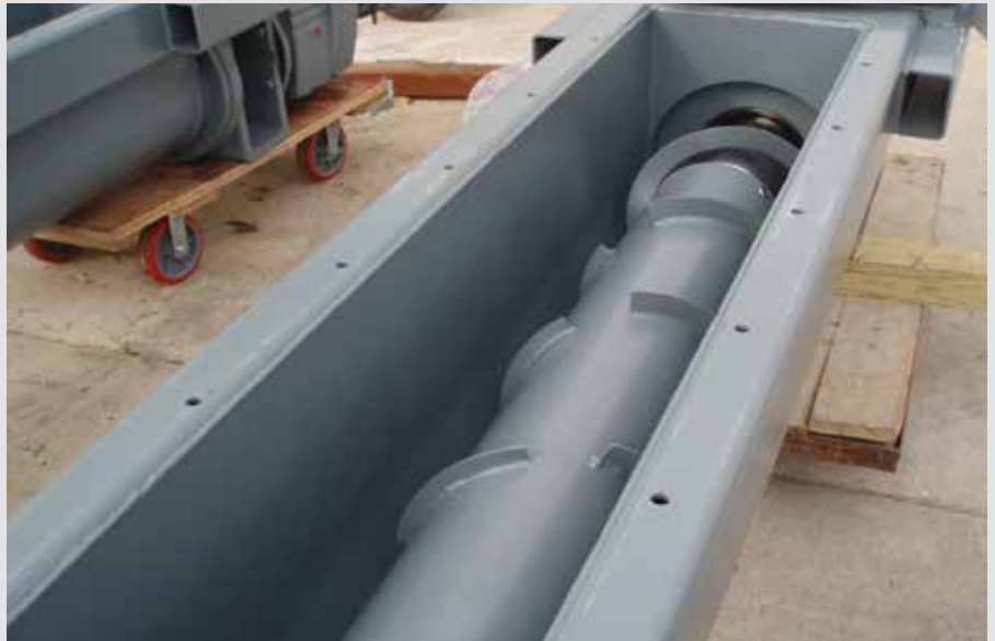
The NETZSCH progressing cavity pump seen here with the segmented, oversized auger with the patented positioned feed screw auger.
