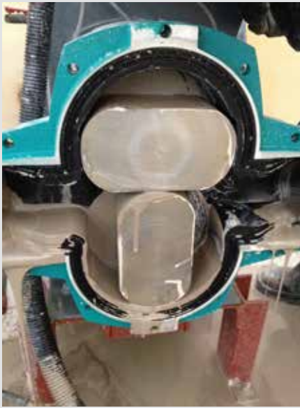
The NETZSCH TORNADO® T2 Rotary Lobe Pump demonstrates Full-Service-In-Place for simple and fast access without disconnecting piping.
