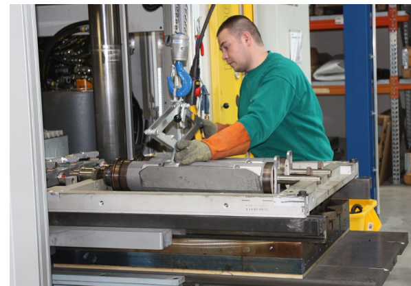
Injection moulding machine for iFD-stators®
