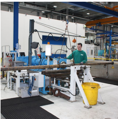
Extruder with stator for oil production
