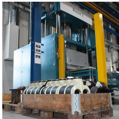
Press with casing liners for TORNADO® T2
