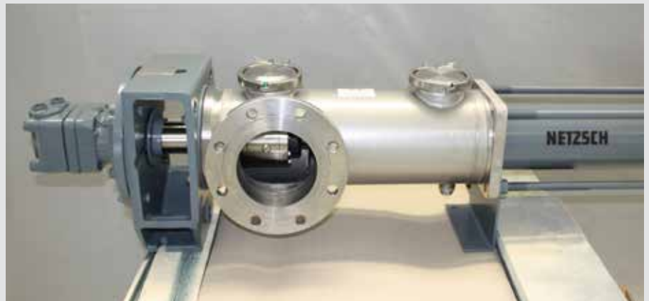
The two inspection openings which have been incorporated above the joints of the coupling rod are the greatest difference with respect to conventional systems. These mean that it is possible to check whether the joints are still sufficiently lubricated and the seals are still intact while the pump is in operation.
