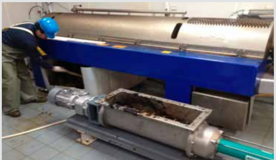
In the seaweed extract application, the NETZSCH pump was installed with a custom flanged hopper to connect to the centrifuge discharge, which conveys the end product into totes.
