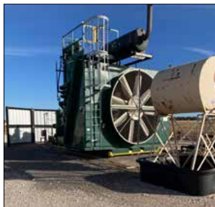
Compressor used to re-inject the gas into the well bore to force the fluids to the surface.
