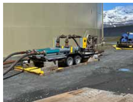
NEMO® Progressing Cavity Pumps easily transfer the high viscosity mix with limited vapor emission
