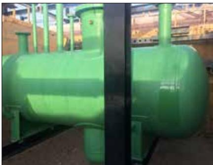
Typical horizontal knockout drum
