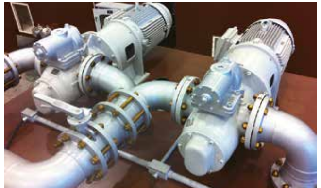
NOTOS® pumps to transfer lube oil to bearings
