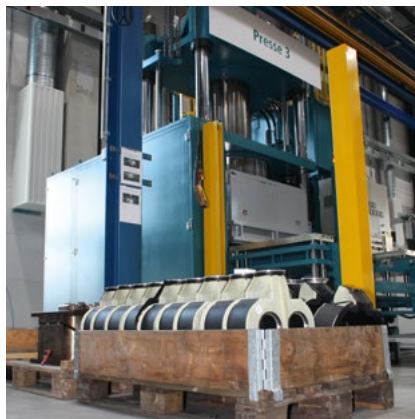
Press with casing liners for TORNADO® T2
