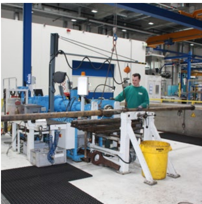
Extruder with stator for oil production
