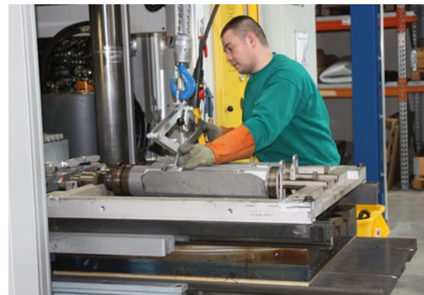
Injection moulding machine for iFD-stators®
