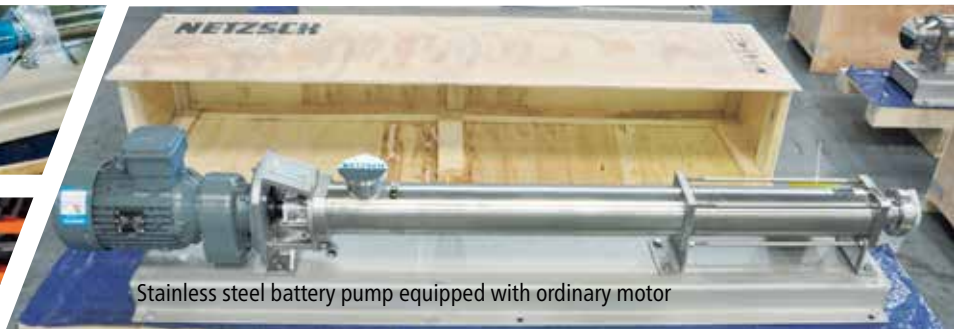
Battery pump with white motor customized according to customer requirements
