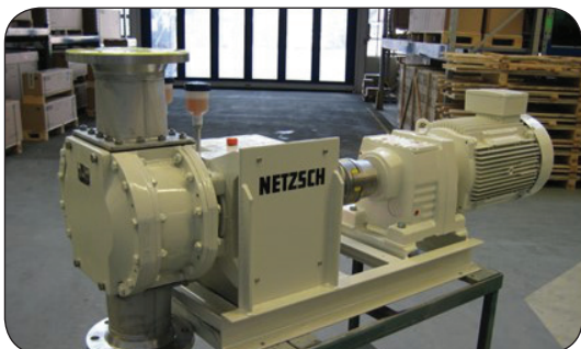
Customized design TORNADO® T1 Rotary Lobe Pump transferring china clay
