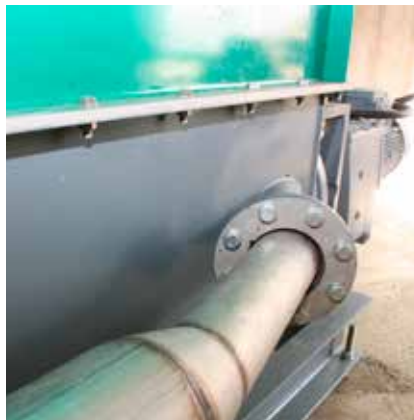
For improved substrate mixing, the entry of the liquid is from the opposite direction of the solids to insure the lengthiest mixing time.
