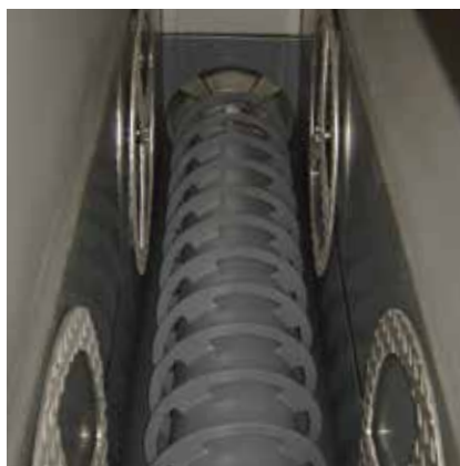
Internal view of the NEMO® progressing cavity pump: Attachment with aBP-Module® to prevent the bridging of sludge cake
