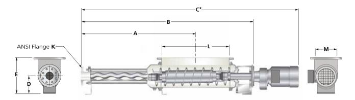
Flow rates up to  $880 \text{ gpm} / 200 \text{ m}^3/\text{h}$  at pressures up to 720 psi / 48 bar.
