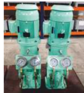
Twin - screw pump for lubricating oil transfer
