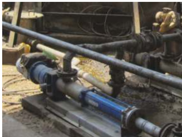
Centrifuge feed using NEMO® BY Pump
