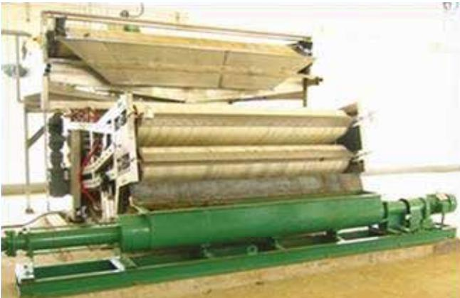
NEMO® Sludge Cake Pump with a 2 meter hopper design underneath a belt filter press conveying sludge 120 ft (37 m) to the drying plant. Solids content is approximately 20%, flow-rate of 26 gpm (6 m<sup>3</sup>/hr) at 120 psi (8 bar) discharge pressure.
