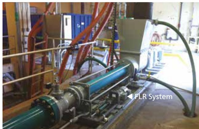
NEMO<sup>®</sup> Sludge Cake Pump with NETZSCH FLR System injecting 0.5 gpm (.11 m<sup>3</sup>/hr) of water into the pipeline to reduce pressures by about 50%. Dewatered sludge is conveyed over 75 ft (23 m) at 15–20 gpm (3.5–4.5 m<sup>3</sup>/hr). Additional flanges added to the hopper for cleaning of the pipeline and pump.
