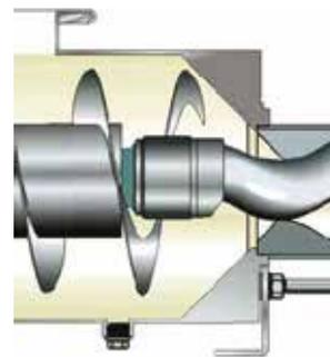
Coupling rod with patented, positioned feed screw to eliminate dead space within the housing and to increase efficiency.
