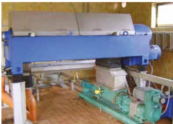
NEMO<sup>®</sup> Sludge Cake Pump being used underneath a centrifuge to convey dewatered sludge over 137 ft (42 m) to transport truck. Solids content approximately 18%, flow rate of 2–3 gpm (.45–.7 m<sup>3</sup>/hr) at 30 psi (2 bar) discharge pressure.
