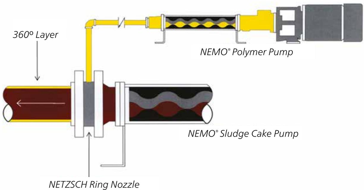
The NETZSCH Friction Loss Reduction System can help you to achieve considerable reductions in pressure, cutting back on operating costs and improving the overall lifetime of your entire system. Pressures over 1,000 psi (70 bar) are easily handled by the NEMO® Sludge Cake Pump when paired with the NETZSCH FLR System. Within the NETZSCH FLR System
