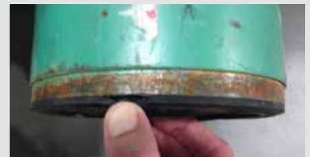
Original NETZSCH part, top Pirate part, bottom
