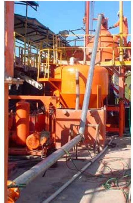
NETZSCH, the global leader in progressing cavity pump technology and sales has produced a cuttings pump to improve the solids control of the drilling fluid recovery of the VCD. This pump makes it possible to efficiently transfer drill cuttings from the shaker or from a holding vessel to the VCD.
