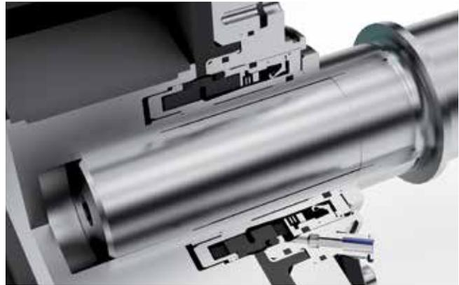
Single acting seal for buffer or quench liquid
