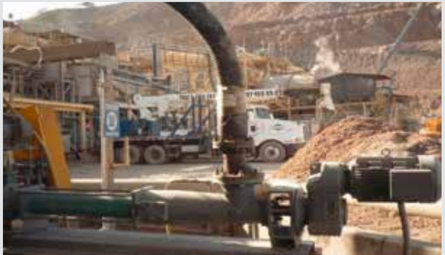
One of the three NETZSCH NEMO® progressing cavity pumps at the mining operation seen here in slurry transport service.
