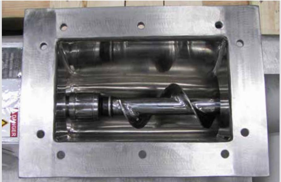
Polished inlet hopper with feed screw.
