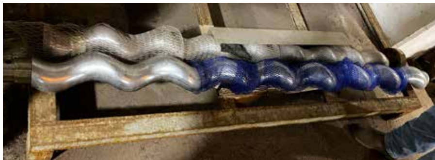
Picture of the pirate rotor part and the previously used original NETZSCH rotor to be replaced after many years of service. The pirate part was the wrong length and had the wrong joint head, therefore it would not fit.
