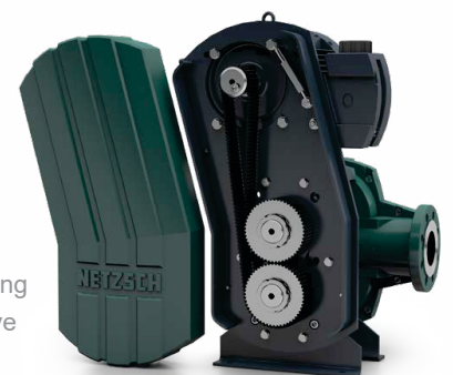
TORNADO ® T2 Rubber-Metal Pump seen from behind: uses a robust and maintenance friendly tooth belt drive
