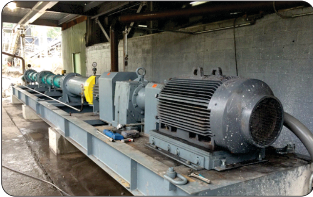
NEMO® Progressing Cavity Pump for coal slurry transfer
