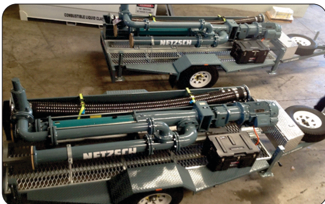
NEMO® Progressing Cavity Pump on Trailer for dewatering application
